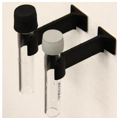
2 pav. \text{NO}_2 , \text{O}_3 pasyvus sorbentas
